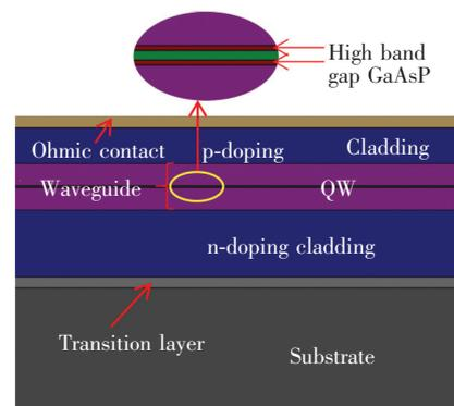
Fig. 1 Schematic of epitaxial structure
