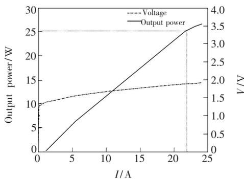
Fig. 4 CW power-current-voltage property of ridge waveguide laser at room temperature
