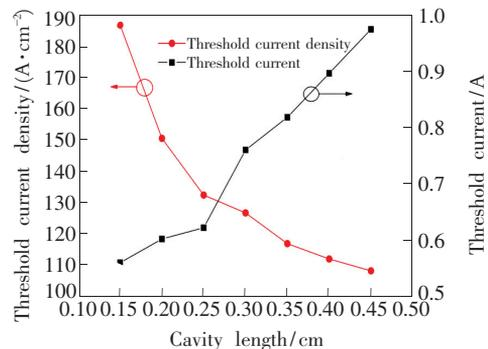
Fig. 3 Threshold current and threshold current density as a function of cavity length
