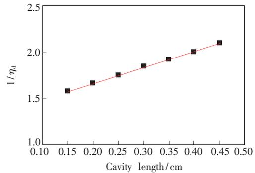
Fig. 2 Picture of inverse external differential quantum efficiency versus cavity length
